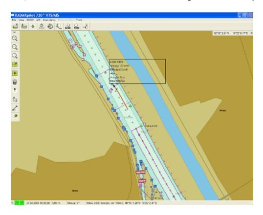
In spring 2005, in-innnovative navigation GmbH delivered system components for the second phase of the project DoRIS (**Do**nau **R**iver Information **S**ervices). RADAR *pilot720°* VTS/AIS is put into operation as surveillance system of the entire course of the Danube in Austria, after successfully testing and optimising the system near Vienna, between the locks of Freudenau and Greifenstein.
