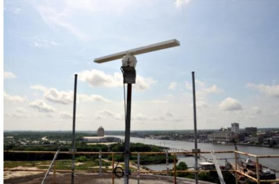
position and velocity of all objects on the river. Radar data are transmitted via DSL from harbor to the VTS display located at the building of Georgia Tech.
