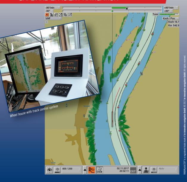
Guiding lines of the integrated navigation system **RADAR** *pilot720*° have to date acted as optical provisions for the ship's route on the waterway. They predominantly consist of curves that adapt themselves to the naturally curved river. The ship's captain can choose the appropriate guiding line from a selection and easily and quickly adjust existing lines directly on the display, as well as create and save new guidelines.
