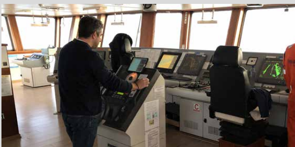
▲ The iPad has a ruggedized case with a handle and can either be placed on the bridge or held by the pilot, for example when mooring.
