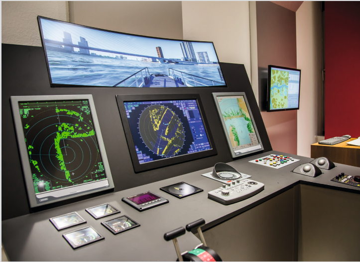
Navigation radar training with 3D visualization at a bridge driven by inVNE ▲
